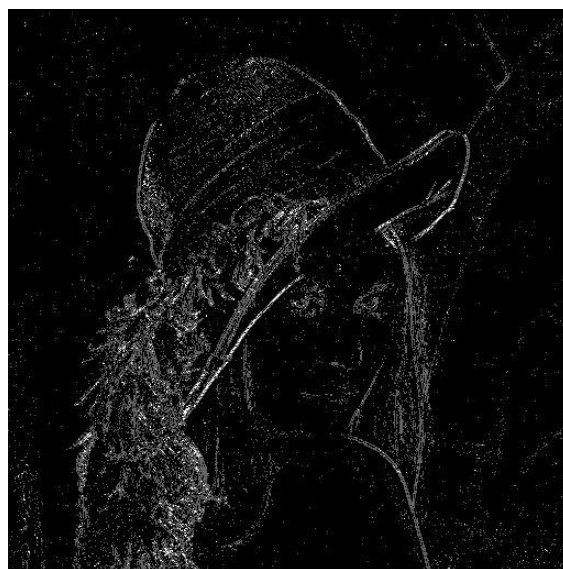
Picture 3. Segmentation of Lenna image. (3 colors used for different segment types: black, grey and bright)
