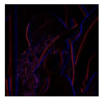
$\underline{Picture3}$ . Sobel 5x5 X-Gradient matrix
