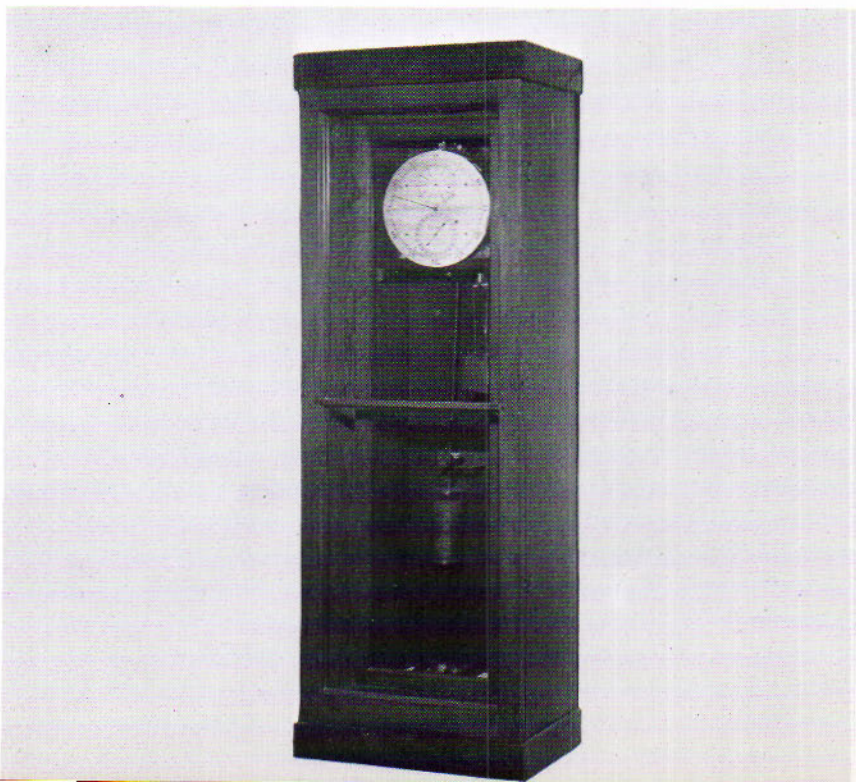
Figure 3.3 A pendulum sidereal clock. The perfection of the pendulum clock was an early major advance in timekeeping. The model here was built by Parkinson and Frodsham. (Photograph by H. Bluemel)
