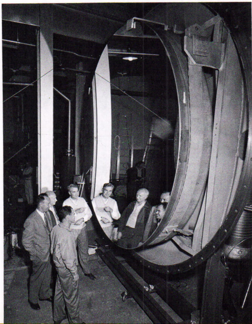
Figure 4.25 The 120-inch (305 cm) mirror just being removed from its aluminizing tank. ( Lick Ob- servatory Photograph. )
