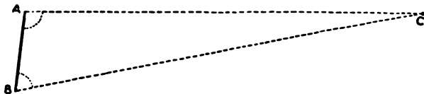
FIG. 44.— Measure of the Distance of an Inaccessible Object by Triangulation.
